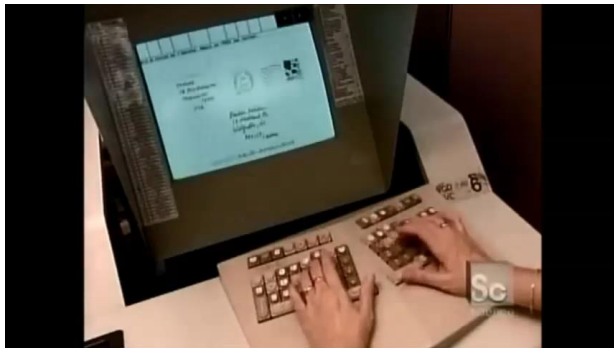
Remote Encoding Centers (REC): Manual keying of mail not read by machines. (click image for video)
